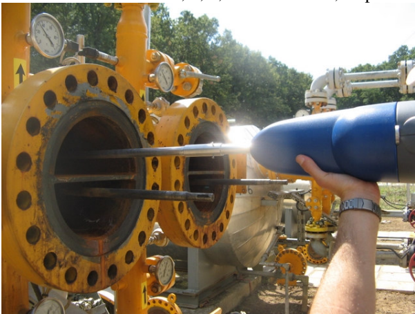
Figure 7 – the probe with the extension tube, inserted into one of the bundles.
