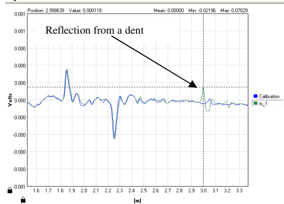
Figure 6: Measurement of u-tube with a dent on the leg beyond the bend, on top of a measurement from a blank tube.
